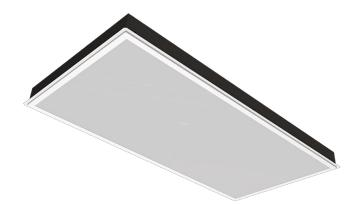
The Tegra LED panel is a bespoke modular luminaire designed to fit in to SAS130 ceilings. The body is made from powder coated steel giving a screwless appearance from under the ceiling. The diffuser is made from high efficiency PMMA which gives the luminaire optimum performance.
