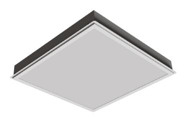
The Tegra LED panel is a bespoke modular luminaire designed to fit in to all SAS130 ceilings. The body is made from powder coated steel giving a screwless appearance from under the ceiling. The diffuser is made from high efficiency PMMA which gives the luminaire optimum performance.
