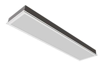
The Tegra LED panel is a bespoke modular luminaire designed to fit in to SAS130 ceilings. The body is made from powder coated steel giving a screwless appearance from under the ceiling. The diffuser is made from high efficiency PMMA which gives the luminaire optimum performance.
